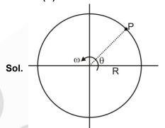
As the particle in uniform circular motion experiences only centripetal acceleration of magnitude  $\omega^2 R$  or  $\frac{v^2}{R}$  directed towards centre so from diagram.
