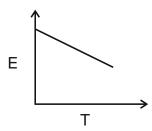
Higher the value of slope  $\left(\frac{\partial E}{\partial T}\right)_P$ , more the deviation between E and E°. Thus, half cell with least value of  $\left(\frac{\partial E}{\partial T}\right)_P$  can be used as reference electrode.
