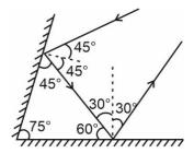
On first reflection angel of deviation is 90° and on second reflection angle of deviation is 120°
