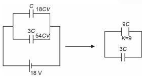
$$V_{\text{common}} = \frac{18CV + 54CV}{3C + 9C} = 6 \text{ V}$$
